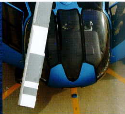
High Visibility blade paint scheme
